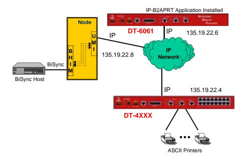
In the above diagram the IP-B2APRT application addresses both the ASCII printer and the BNS circuit group for each particular printer. The operation is similar to the BNS A2B DKAP with regard to the printer functionality.
